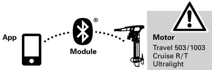
TorqTrac uses the energy-efficient Bluetooth® Low Energy (BLE / Bluetooth® LE) for data transmission. To use this technology, your device must meet certain requirements. Please ask the manufacturer of your device to be sure that Bluetooth® Low Energy is supported.
