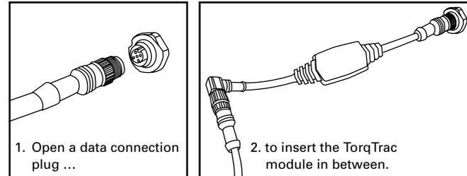
**Note:** To ensure a stable data connection via Bluetooth® SMART, make sure that the TorqTrac module is always plugged in as close as possible to the tiller or remote throttle control.
